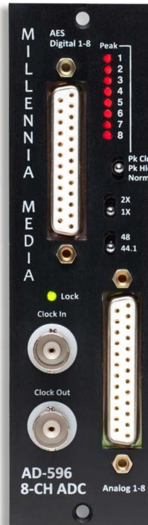
**DB25 Connectors** conform to the Tascam pin out. Please note you can't use a pin to pin DB25 cable to connect the digital outputs to a DB25 digital input connector. A special cross cable is required.
