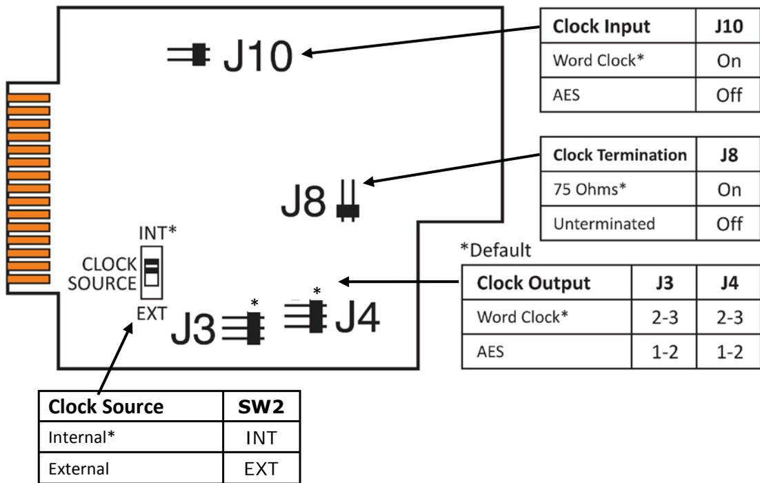
The **Clock Source** switch is accessible without removing the cover.
